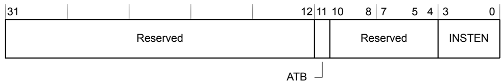
Figure 13-5 TRCEVENTCTL1R bit assignments
