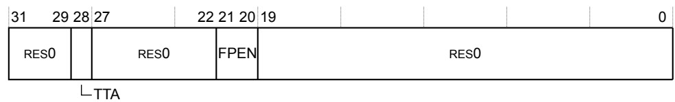
Figure 4-29 CPACR_EL1 bit assignments
